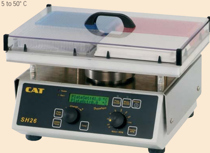
SH26 Heating Shaker for 4 MTP's (horizontal circular motion) Operating temperature range roomtemperature to 90°C or 120°C Shaking frequency: 50-1100 rpm
