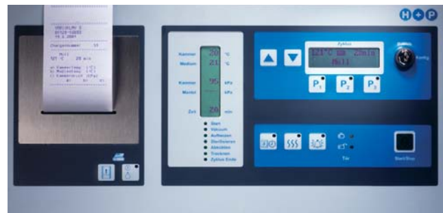
START / STOP key on the control panel opens and closes the swing door
