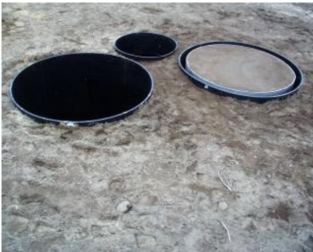
Implanting the lysimeter vessels in the station
