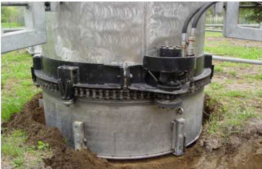
Lysimeter vessel with soil milling
