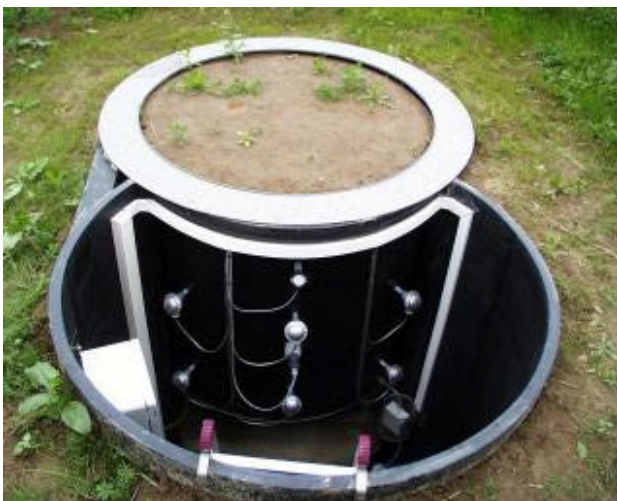
Weighable lysimeter with soil hydrological sensors
