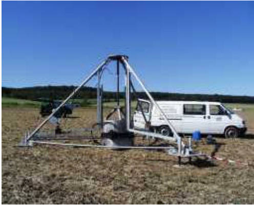
Lysimeter excavation System
