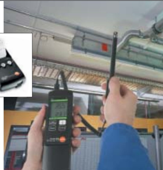
Measures the ambient moisture at the outlet of an air conditioning unit
