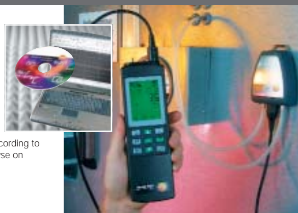
Monitors filters using the external 100 Pa probe
