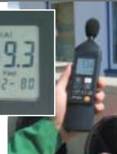
testo 815, Monitoring measurements on ventilation
