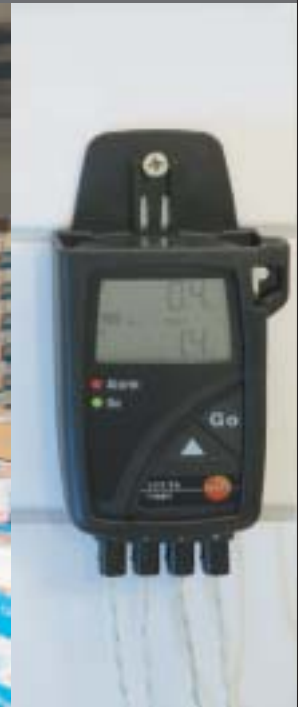
Simultaneous temperature measurement at up to 4 different locations
