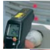
830-T2, 2 point laser sighting (real measurement point)
