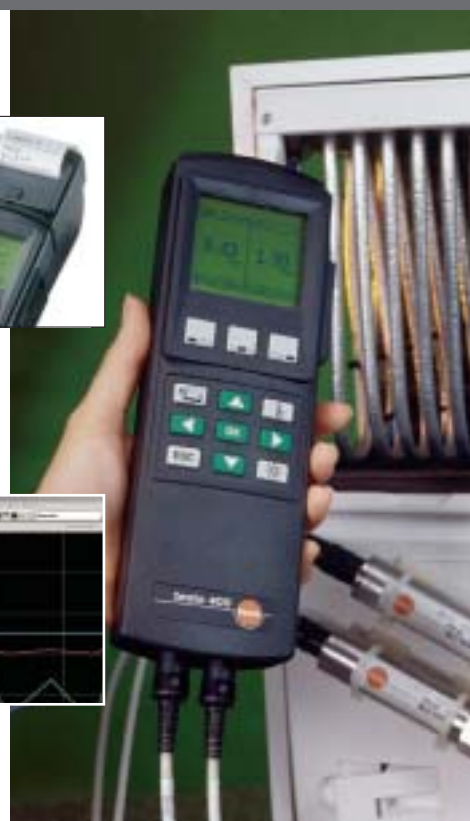
Measurement on a refrigeration machine, low/high pressure
