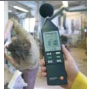
testo 816, Checking noise control
