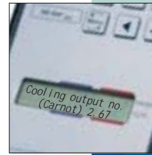
Display of calculated Carnot and Lorenz cooling/heating output figures
