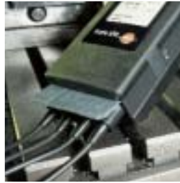
Connection option for up to 4 ambient air probes per logger
