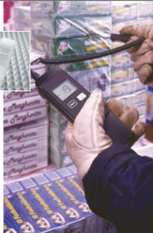
Temperature measurement in refrigerated store rooms or cabinets.
