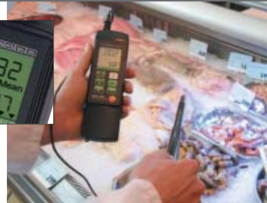
Monitors air circulation in a refrigeration cabinet
