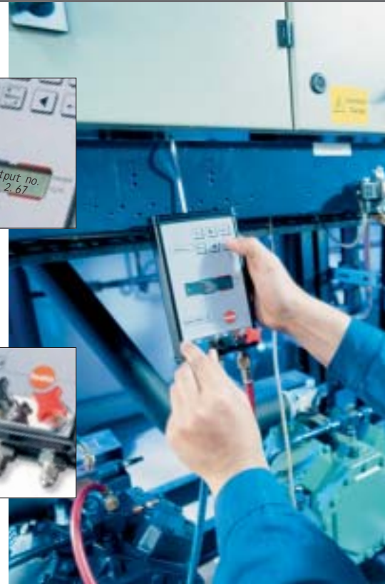
Determining vaporisation and condensation temperatures
