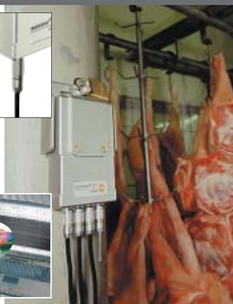
Monitor several refrigerated storerooms using testostor 171-4
