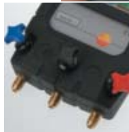
Valve bank, back pressure, high pressure, filling, disposing
