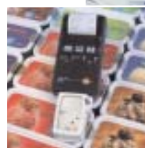
testo 177-T1 without display, data is printed on site on the fast testo 575 printer
